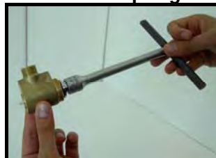
5 - undo the cartridge
