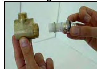
6 - remove and replace the cartridge
