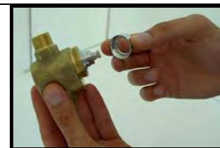
8 - ring nut in upside down position
