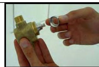
8 - ring nut in upside down position
