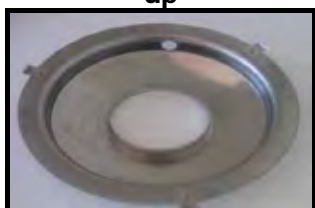
11 - upper pan with the three clips already assembled
