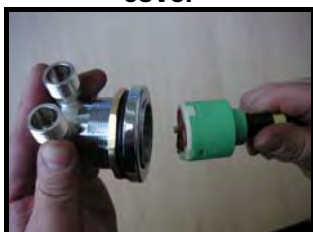
19 - remove the cartridge
